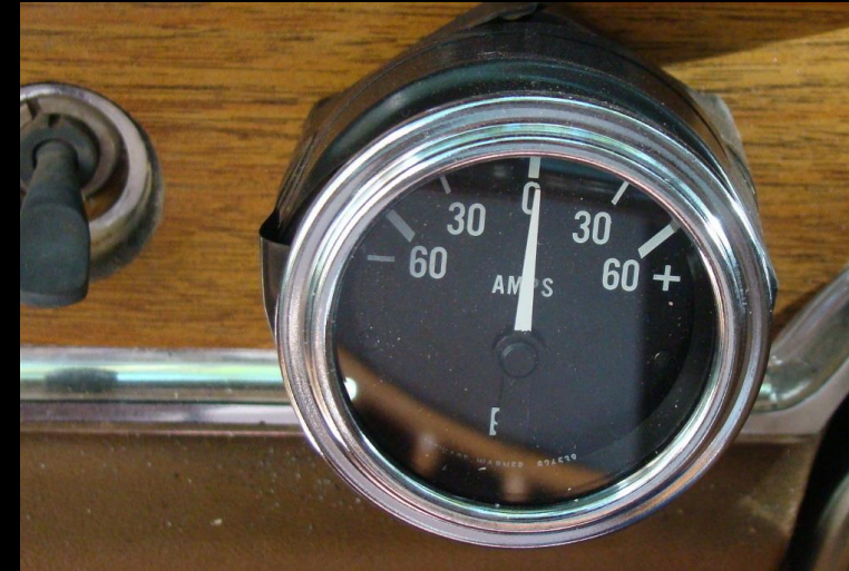
Added generator AMPS meter
