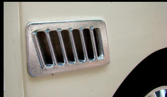
Added engine vents
