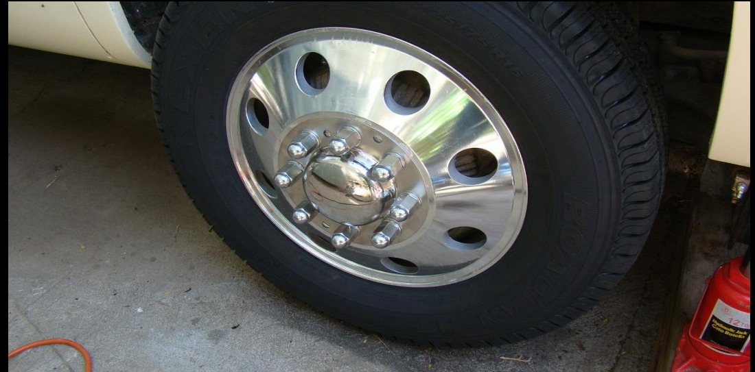
I purchased the six aluminum wheels with the new tires. They were mounted, balanced, driven some number of miles and then trued to roundness prior to shipping.
